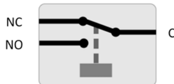
Internal operation of the programmable relay
