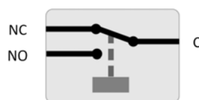
Relay configuration (not energised).
